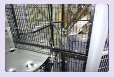
For this particular project a foldable spoon needed to be placed into a cap, which is supplied to a manufacturer of milk-based fast foods. A disposable plastic spoon is very difficult to orient due to the design of the moulding, especially at 120 parts per minute.
